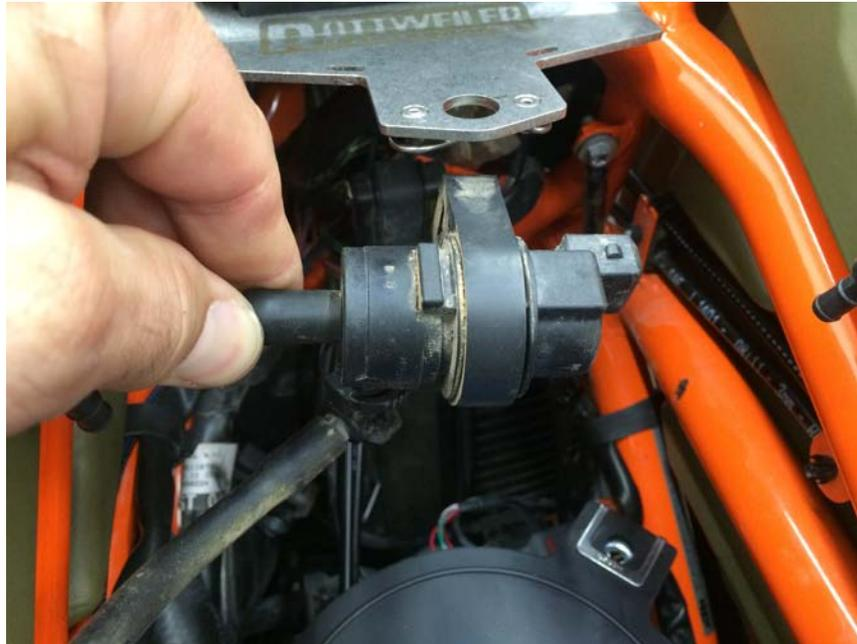
This is the typical routing of the canister lines.
