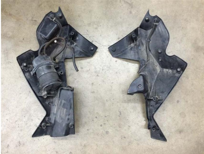
In the stage 3 kit, the Tygon hose will now loop up and then down inside the inner fairing as shown below on the Adventure 950/990.
